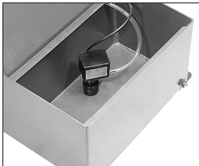
**Figure 14.** Coolant pump.
